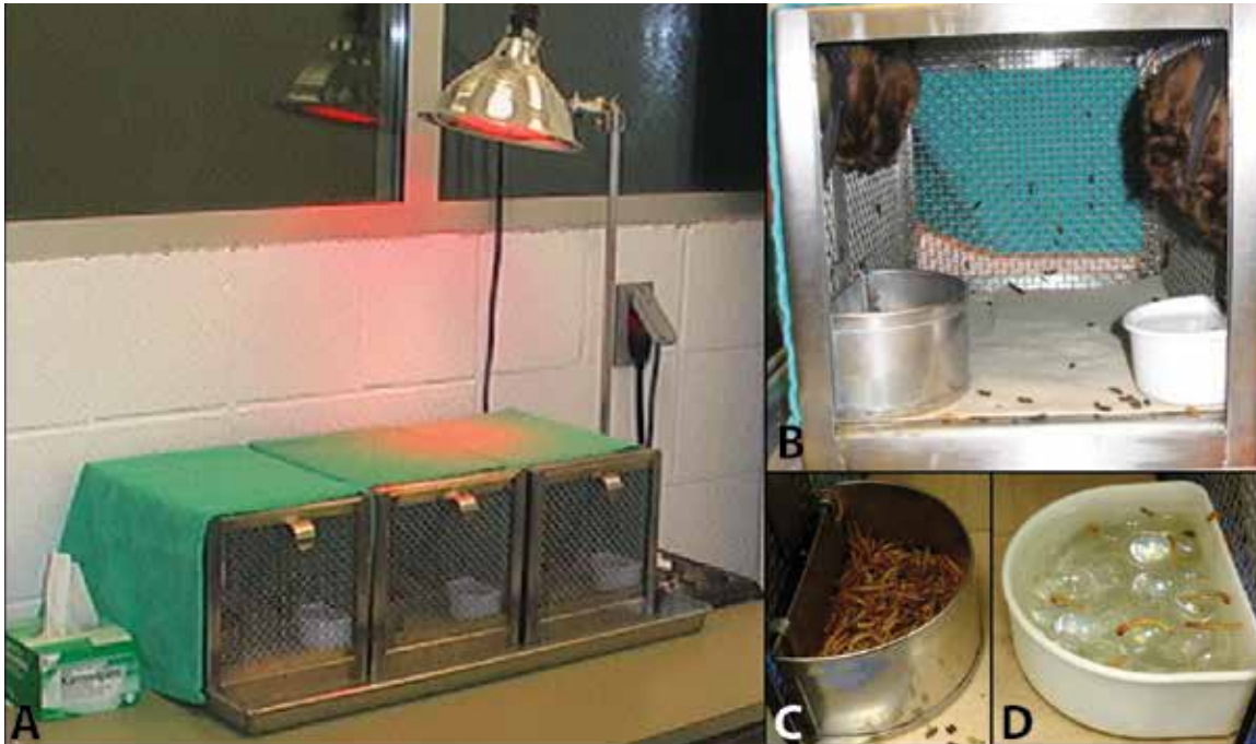
Figure 8A-D. Small cages for Eptesicus are kept at the desired temperature by a heat lamp (A, B) and contain mealworm (C) and water containers (D). To prevent drowning, the water container is partially filled with large glass beads.
